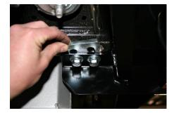
18. In behind mud in wheel arch, fit M12 bolt on wire through hole in chassis, down to side plate in Kaymar bar, secure using M12 flat, spring and nut. Do this to either side. **DO NOT TIGHTEN**.
